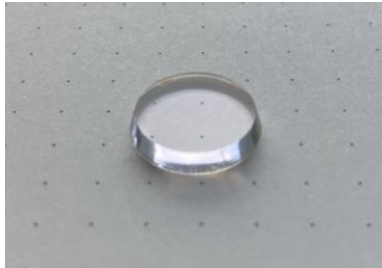
Figure 1. A photograph of a polished 2.0 at.% \text{Er}:\text{Na}_5\text{Y}_9\text{F}_{32} crystal.
