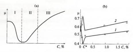
Fig. 1. (a) The general dependence of the dynamic coefficient of friction  $\mu$  on the concentration C, % of the surfactant on the fiber surface; (b) *1*—change in the dynamic coefficient of friction; *2*—change in the coefficient of tangential resistance;  $C^*$ —concentration corresponding to the formation of a monomolecular layer.
