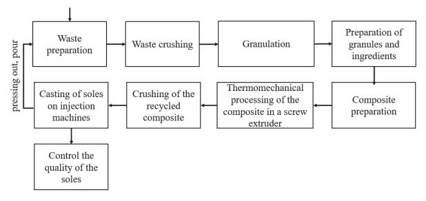
FIGURE 3. Technology for producing compositions for the sole of shoes with a fibrous filler
