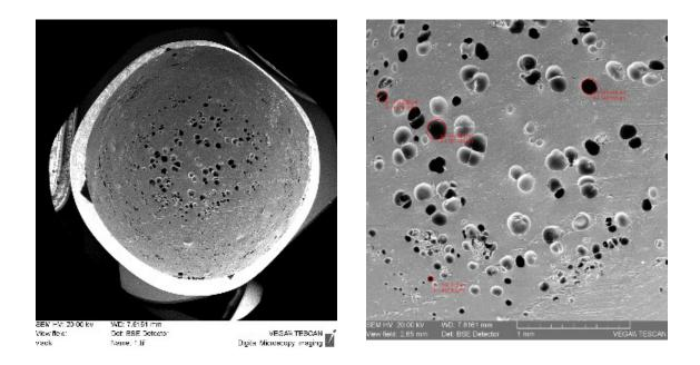
Figure 1 – Porosity of the resulting granulate
