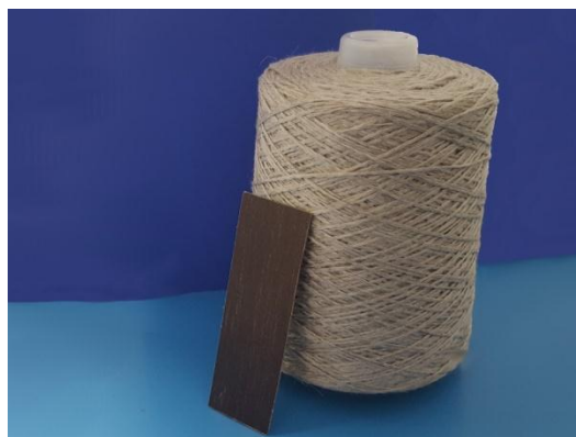
Figure 1 – Prepared linen roving and composite material formed using it
