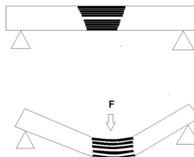
Figure 5 – Concept of the superstable structure based on the package of superelastic beams with completely reversible giant deformation
