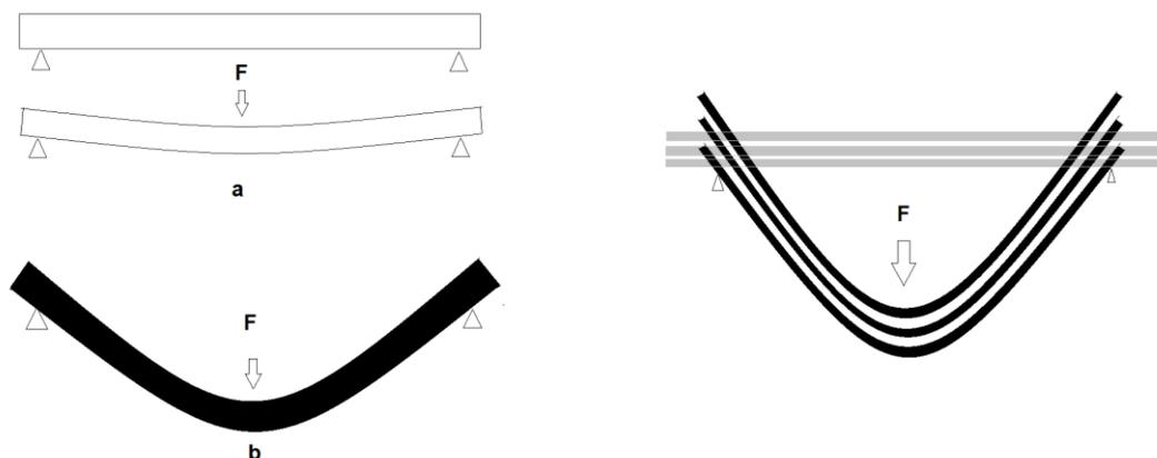
Figure 2 – The concept of giant reversible superelastic deformation: (a) normal elastic deformation of steel; (b) superelastic reversible deformation of the Fe-Ni-Co-(Ta-B) alloy for the design of superstable structures
