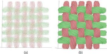
**FIGURE 10.** A section of fabric after modeling the interaction of fibers. (a) - fibers in the form of lines; (b) - fibers in the form of tubes.
