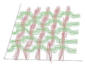
FIGURE 9. Fabric section model
